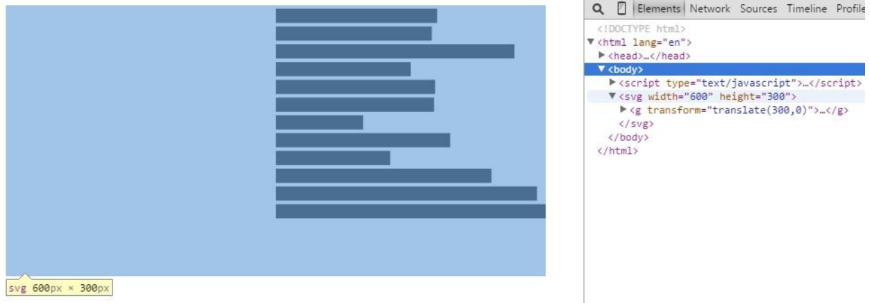
Figure 3. The rectangles are now drawn inside the g element that is contained within the SVG element. Now there is room for labels and an axis (The SVG element is highlighted in the image).
